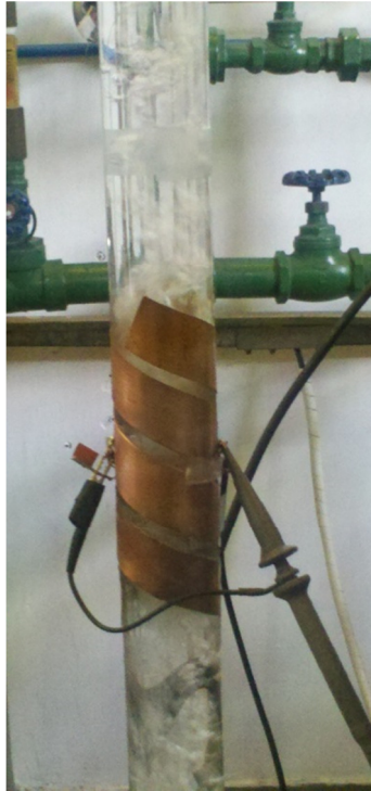
Figure 3. Capacitance sensor flush mounted on test facility.
