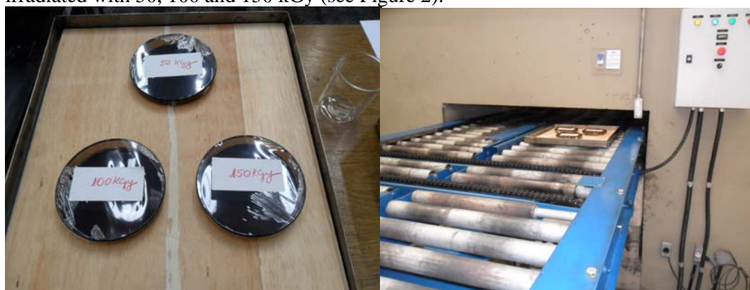
Figure 2: Samples GA11, GA11.1 and GA11.2 poured into the petri dishes to start the electron beam radiation process in a industrial electron accelerator Dynamitron model DC 1500/25-JOB 188.
