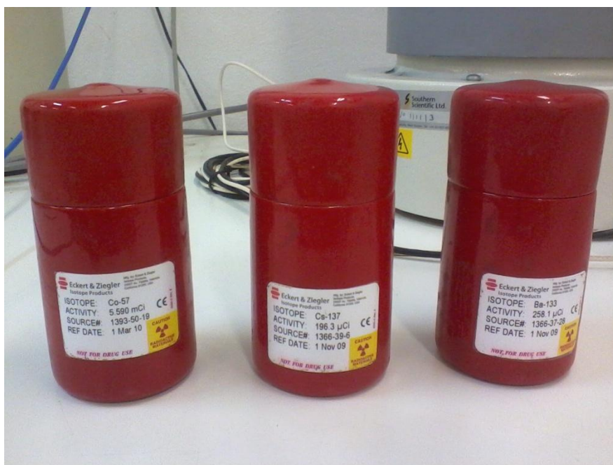
Figure 2: From left to right, ^{57}\text{Co} , ^{137}\text{Cs} and ^{133}\text{Ba} radioactive sources used in this study.
