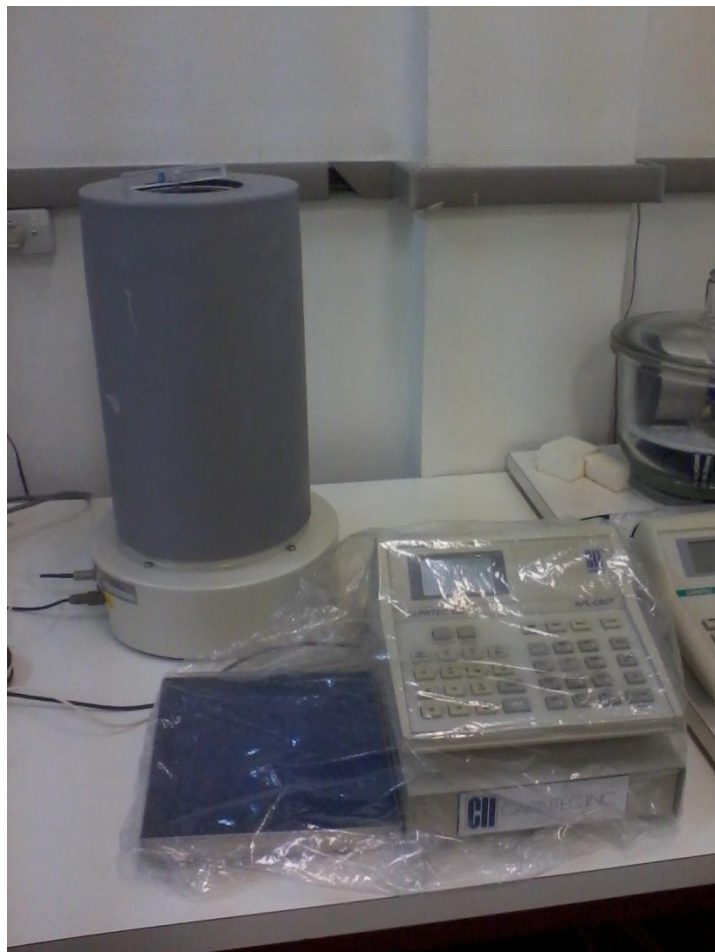
Figure 1: Activity meter Capintec NPL-CRC used in this study.
