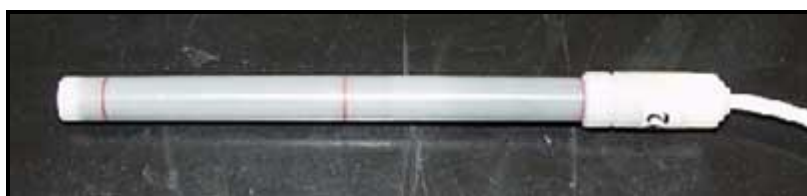
Figure 2: Pencil ionization chamber, Radcal
