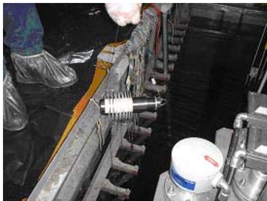
Figure 1. Photograph of rack with vertically oriented coupons being withdrawn from the storage section of the reactor pool.
