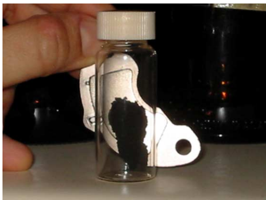
Fig. 4. MnMagBead particles being attracted by a magnet.
