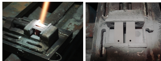
Fig. 1. HVOF deposition process and coated specimens
