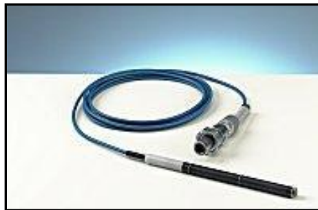
Fig. 2: Calibrated pencil ionization chamber
