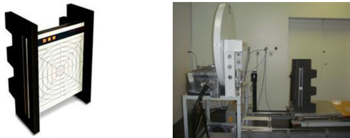
Figure 1. Patient Dose Calibrator and the set up used to measure the parameters
