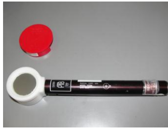
Figure 3. Radcal Ionizing chamber used to test the HVL
