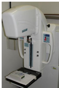
Figure 2. The kVp meter (Diavolt) positioned on the breast support
