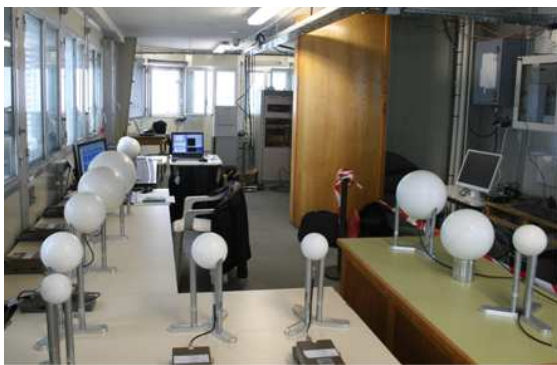
Fig. 2: HERMEIS neutron spectrometer located in the Pic-du-Midi station (altitude, latitude and longitude are respectively equal to 2.885 km, 42°55'N and 0°08'E).
