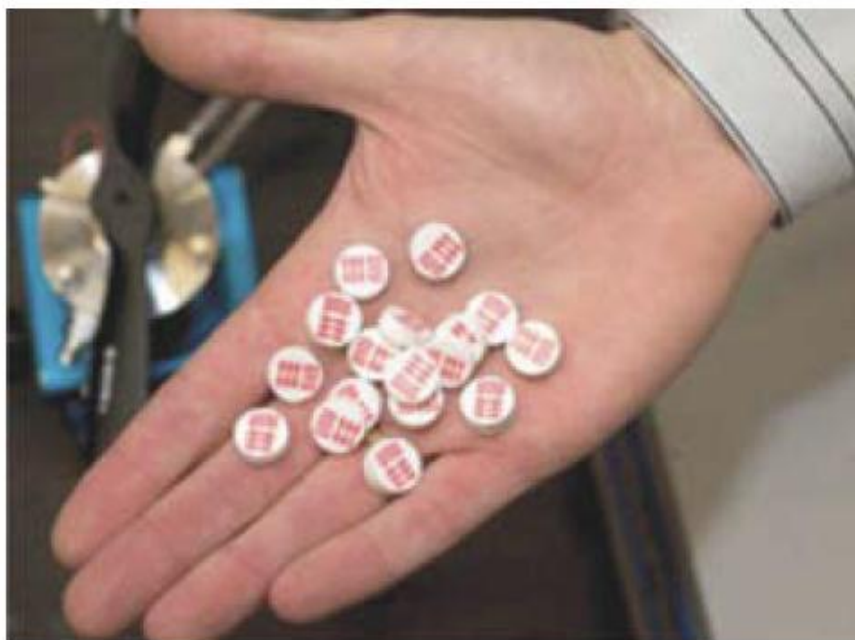
Figure 3. Pellets of \text{Mg}(\text{NH}_3)_6\text{Cl}_2 , a carrier for ammonia. The pellets hold \text{NH}_3 at nearly its density in liquid ammonia, but at a vapor pressure of only 2 mbar; there is no significant release of ammonia to the environment and the pellets can be handled safely. The pellets are charged at room temperature and release ammonia above \sim 100^\circ\text{C} . After Reference 31.
