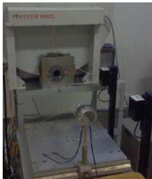
Figure 2. Experimental setup with the tandem ionization chamber system positioned at the calibration distance
