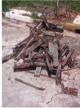
Figure 1: Painted perforated carbon steel structures after the facilities dismantling.
