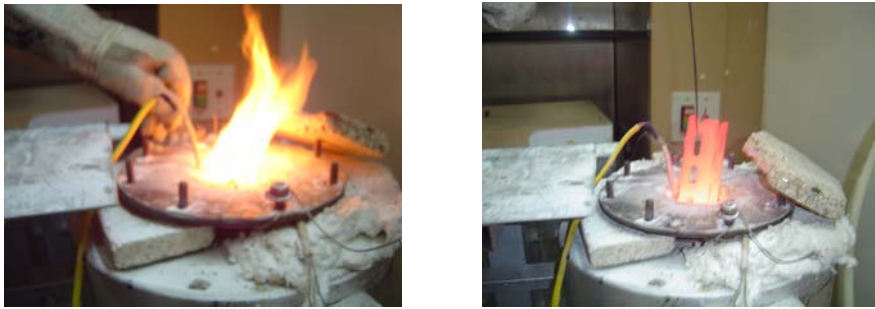
Figure 2: molten salt stripping - introduction (left) and removal (right) of a sample.
