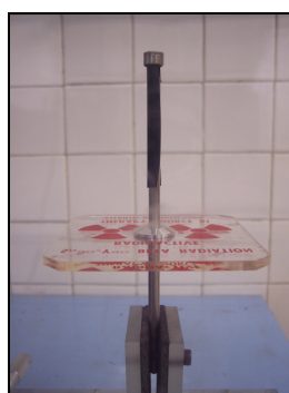
Fig. 1. ^{90}\text{Sr}+^{90}\text{Y} NIST applicator (plane/dermatological source) used in this work as reference in the calibration of the other applicators.
