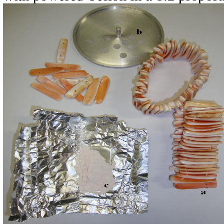
Fig. 1. a) Bracelet made of natural oyster shell; b) pellets of oyster shell powder with Teflon and c) powder of oyster shell on an aluminium foil.
