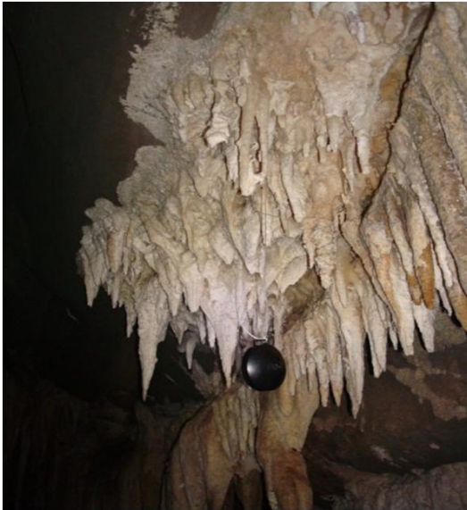
Figure 3. Santana Cave with diffusion chamber and CR-39 inside.
