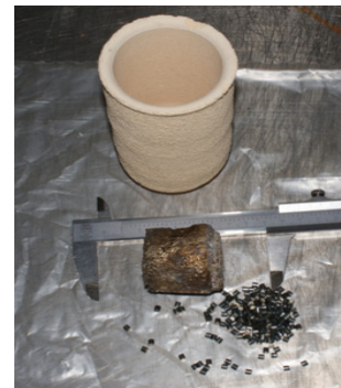
Figure 1 – Uranium ingot, Molybdenum cylinders and Zirconia crucible.
