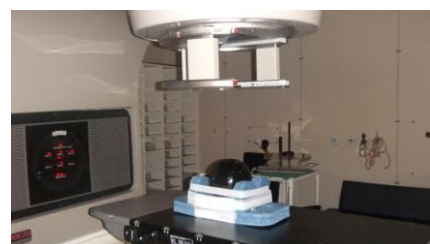
Fig. 2 Experimental set up for FXG spherical phantom irradiation with 6 MV clinical photon beams using a Clinac 600C linear accelerator
