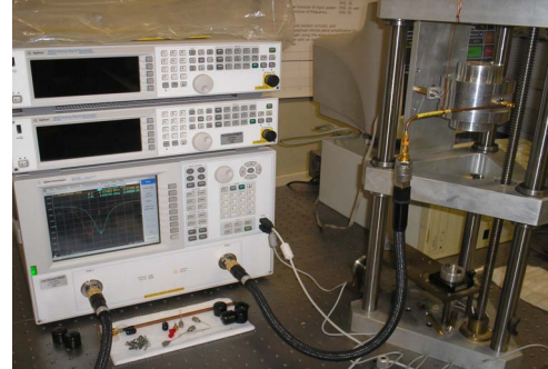
Fig. 5. Experimental apparatus used in the calculation of the cavity R_{sh}/Q_0 using the perturbation method.
