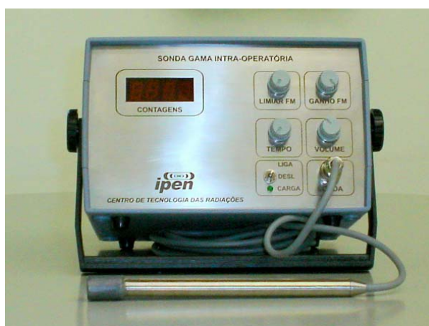
Fig. 2. Probe and counter developed at IPEN.
