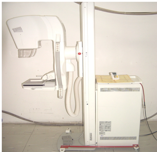
Figure 1: Mammography X-ray equipment model Senographe 700T (GE).
