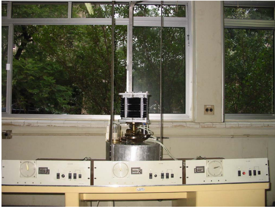
Figure 3. The focusing silicon monochromator ready to be installed in the new diffractometer.
