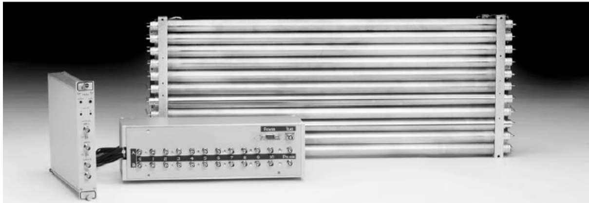
Figure 1. The neutron PSD array, the junction box and one of the linear PSD signal processing electronics elements.
