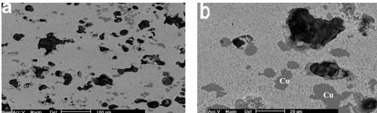
Figure 5: SEM of the alloy W-25w%Cu prepared with mixed powder and sintered at 1200°C for 1 hour. A view of the structure (a) and details of the pores and Cu lakes (b).
