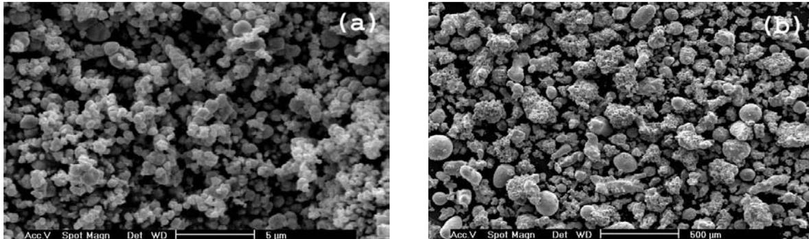
Figure 1: SEM micrographs of the tungsten (a) and copper (b) as supplied powders.
