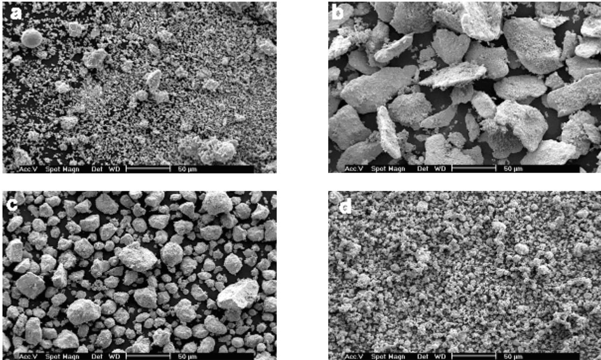
Figure 2: SEM micrographs of W-25w%Cu prepared by mechanical mixture (a) and high energy milling for 2 (b), 50 (c) and 100 (d) hours.
