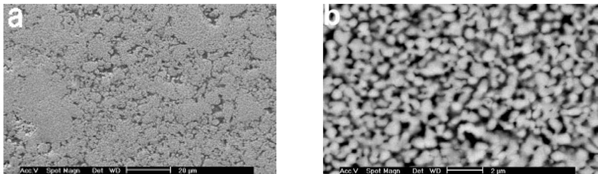
Figure 6: SEM micrographs of the alloy W-25w%Cu sintered at 1200°C for 1 hours. Granulated dense structure (a) and detail of a granule of the structure showing the fine grains of tungsten in a copper matrix (b).
