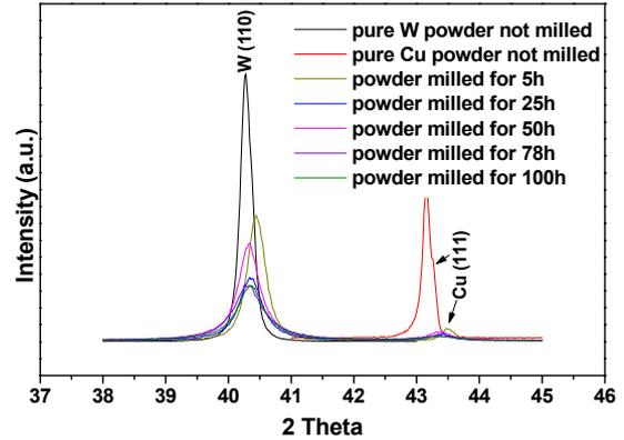
Figure 4: Diffraction peaks of tungsten (110) and copper (111) of powders milled for different times and the hand mixed powder.
