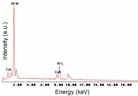
Figure 3: EDX spectrum of the composite W-25w%Cu after 100 hours of milling.
