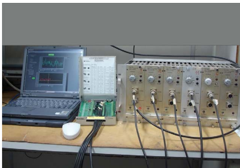
Figure 9. Isolating amplifiers used in the noise analysis methodology.
