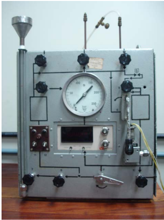
Figure 5. Ramp pressure test equipment.
