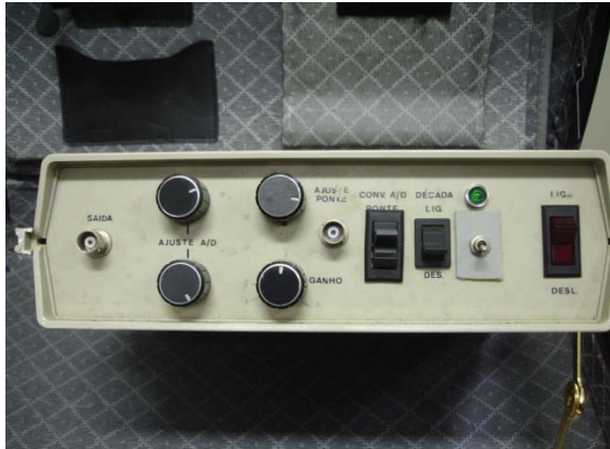
Figure 2. LCSR test equipment.
