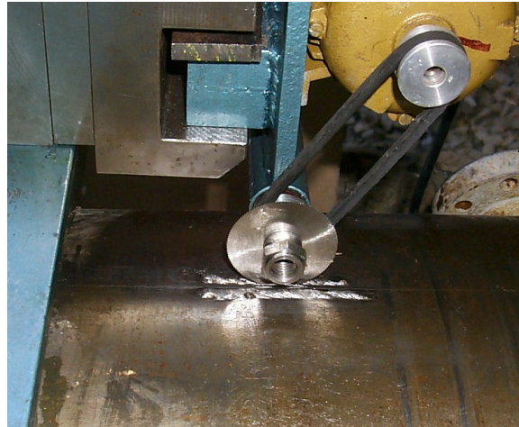
Figure 5 - Notch machining on the vessel model wall
