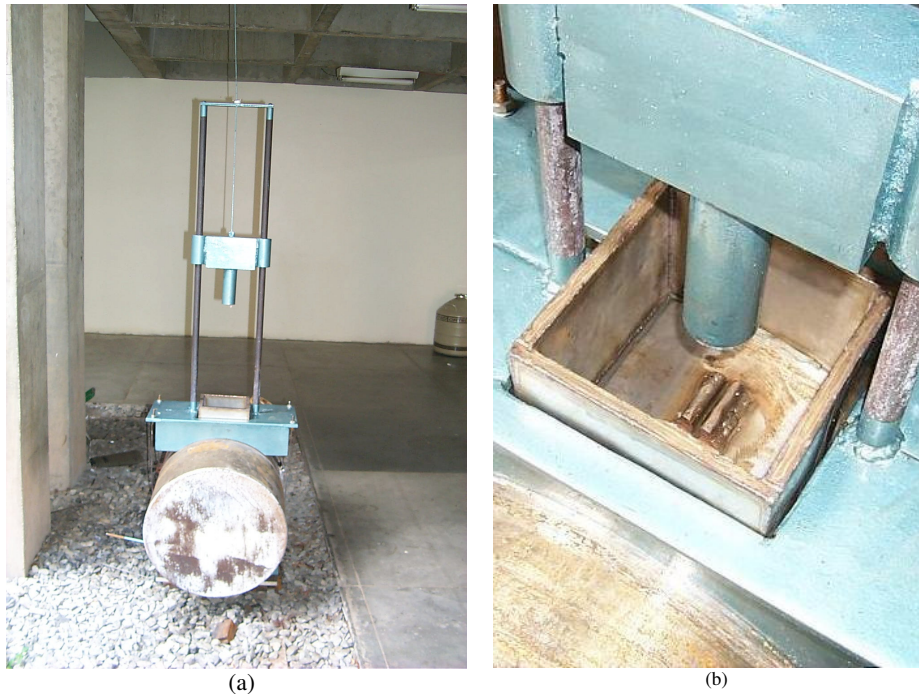
Figure 8- (a)- Drop weight system mounted over the RPV model, (b)- view of the weight positioned over the notch
