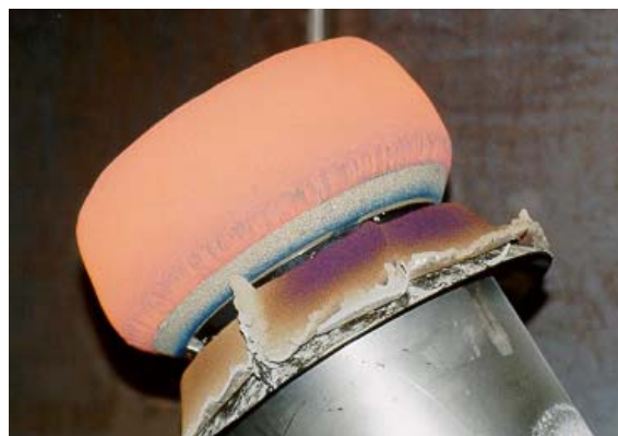
Figure 1. Spray formed AISI M2 obtained in a plant installed at IPEN/SP.
