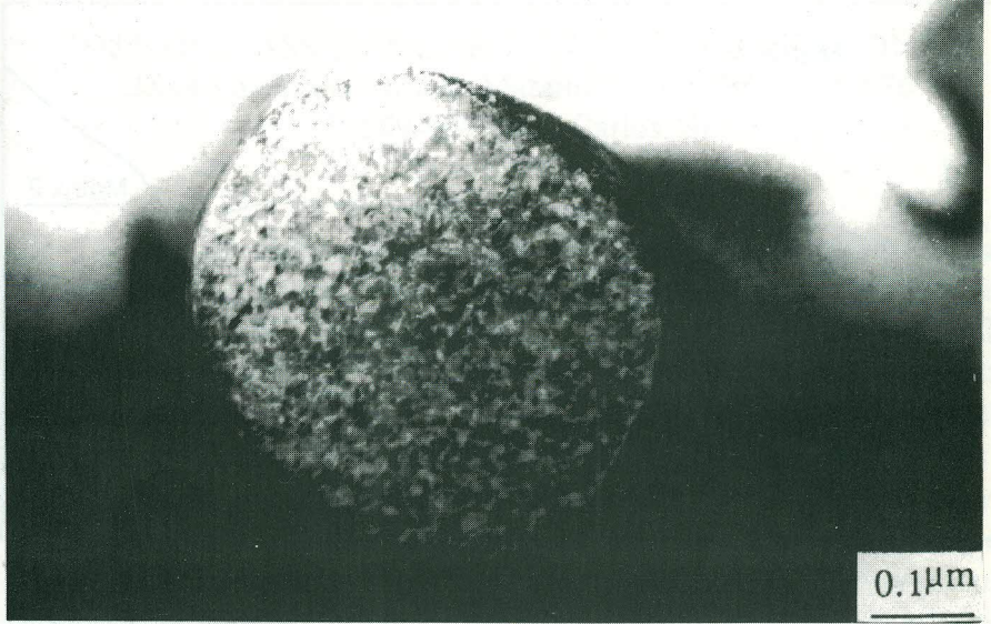
Fig.1 TEM micrograph showing a large Nd 2 O 3 oxide within a matrix grain.
