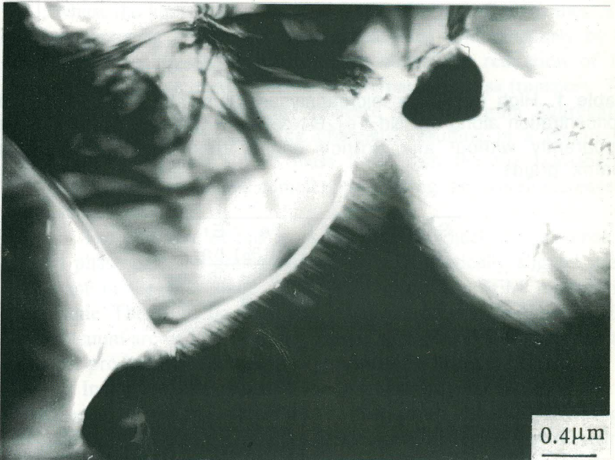
Fig.2 TEM micrograph showing large Nd 2 O 3 oxides at a boundary between the matrix and the boron-rich grain.
