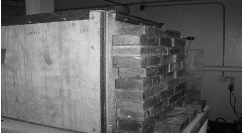
Fig.1 – Exposure cave showing the lead-bismuth bricks in front where enters the neutrons beams coming from NSC Reactor.
