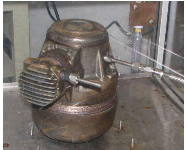
Figure 20 – A CO 2 compressor during the extreme hydrostatic test pressure.
