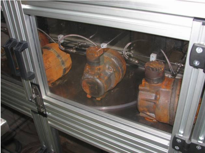
Figure 21 – A fatigue test of the compressor housing running on a special developed machined
