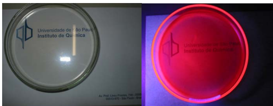
Figure 1 Chitosan Film doped with \text{Eu}^{3+} Chelate.
