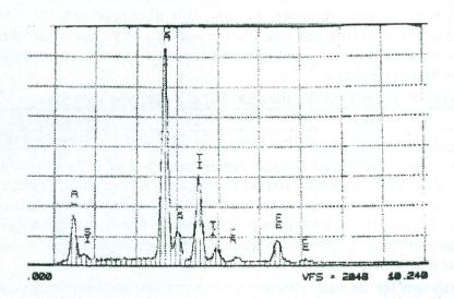
Figure 2: Particle (arrow figure 1.(b)) EDS analysis. Ca rich particle.
