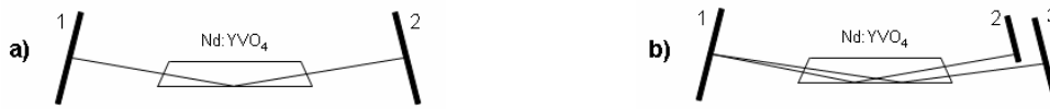
Fig. 1: Cavities configuration: a) Single bounce: 1) end mirror ( R=50\text{cm} ); 2) plane output mirror with 36% transmission; b) Double bounce: 1) folding mirror ( R=50\text{cm} ); 2) high reflector (plane mirror); 3) plane output mirror with 36% transmission.
