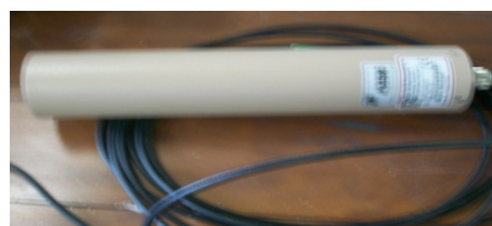
Fig. 3 NaI scintillator of 2'', Ludlum, model 44-10.
