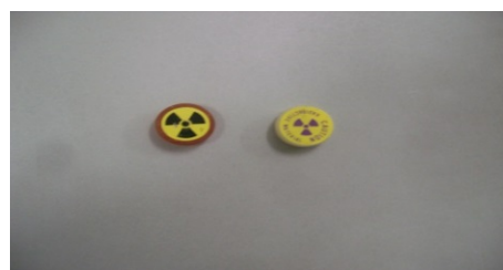
Fig. 2 241 Am (left) and 137 Cs (right) sources.
