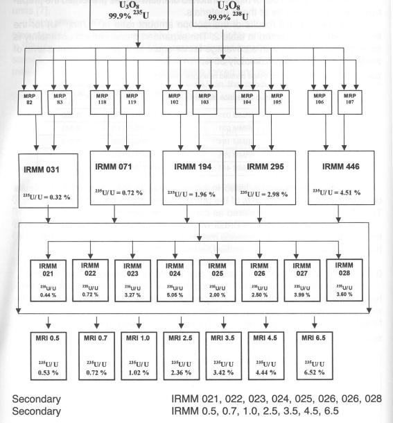
Figure 1 - Metrological traceability chain for uranium samples.
