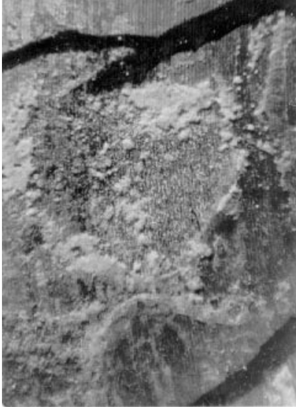
FIG. 5.12. Coupon 6064/64, crevice corrosion (18 ×).
