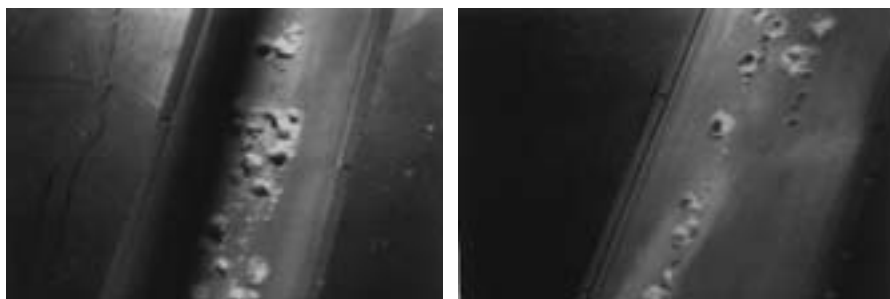
FIG. 1.2. Nodular corrosion products and exposed pits on MTR type spent nuclear fuel.
