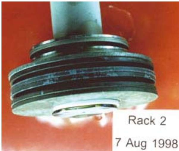
FIG. 13.3. Rack 2 after six months of immersion.
