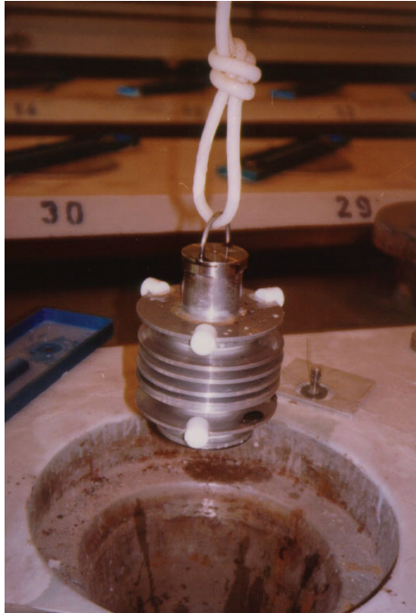
FIG. 5.1. Rack 1 as extracted from channel.
