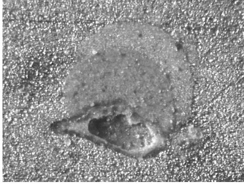
FIG. 5.31. Detailed view of one pit inside the island (20 ×).
