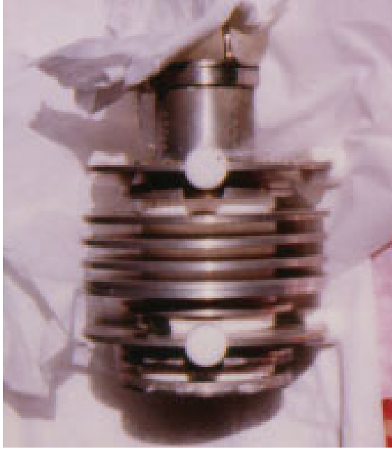
FIG. 5.3. Side view of rack 1 after extraction. Corrosion products can be seen emerging from inside the two galvanic couples at the bottom of the assembly.
