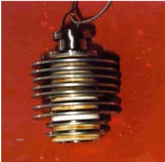
FIG. 9.1. Rack 1 just prior to the second immersion.
