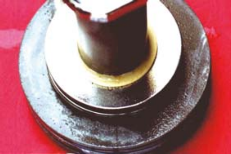
FIG. 13.4. Rack 2. Scratch mark on the 6063 alloy after 24 months of immersion.
