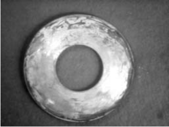
FIG. 8.4. A 6063 coupon from rack 3 after exposure to the basin water for two years.
