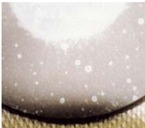
FIG. 1.6. Pitting caused by embedded iron filings.
