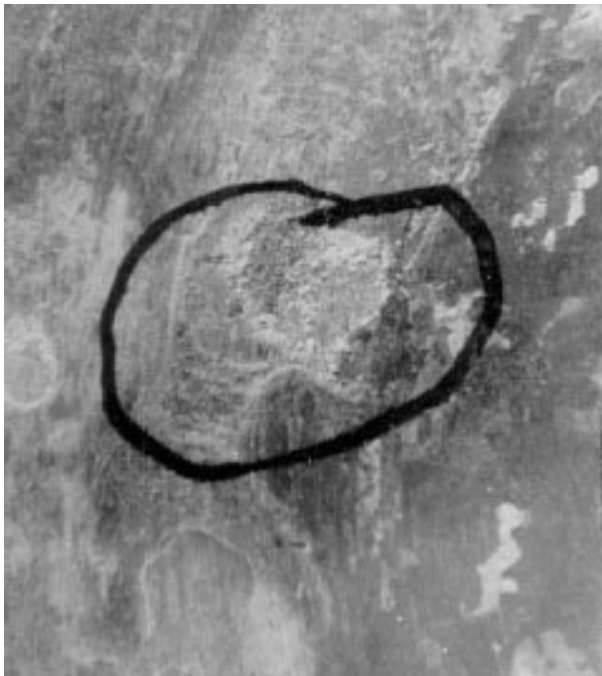
FIG. 5.10. Coupon 6063/64, crevice corrosion (6 ×).
