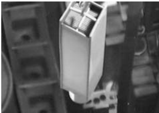
FIG. 1.1. Typical MTR type spent nuclear fuel element.
