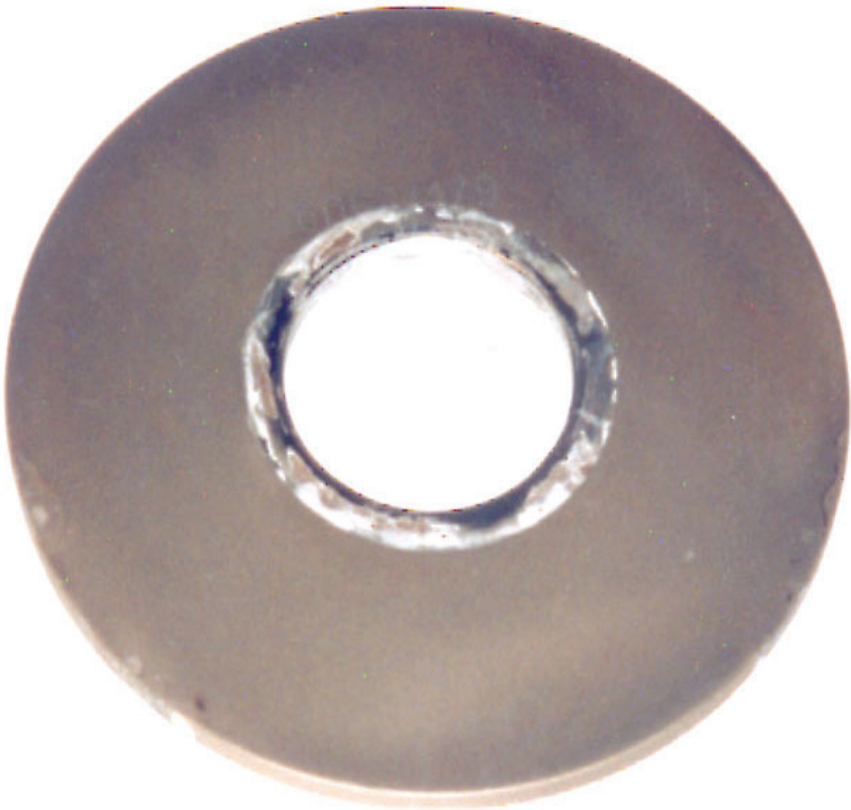
FIG. 5.26. Thick oxide covering surface of sample (1 ×).
