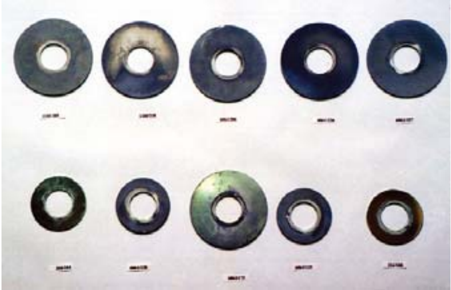
FIG. 7.2. Surfaces of coupons from rack 2.
