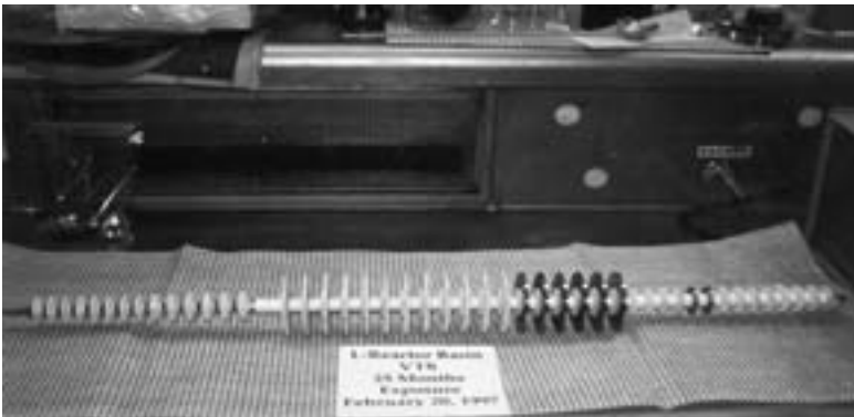
FIG. 1.5. FRR corrosion surveillance rack.
