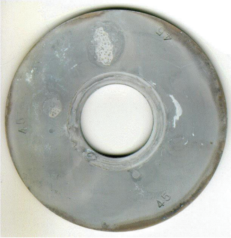
FIG. 5.29. Islands of pits on an otherwise intact sample (1 ×).
