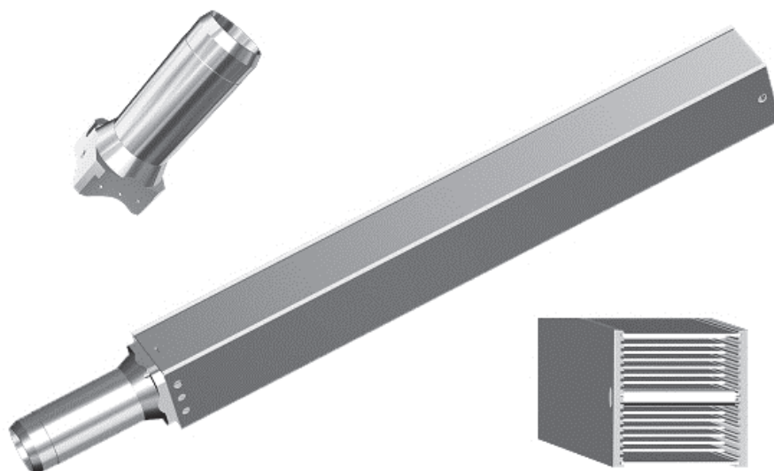
Fig. 16. Schematic illustration of the fuel element produced at IPEN.
