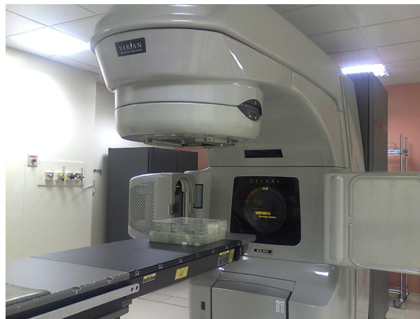
Fig. 1. Varian model Clinac 2100C linear accelerator of the Hospital Israelita Albert Einstein.
