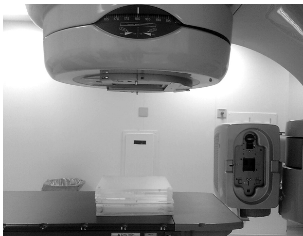
Fig. 2. PMMA phantom and TLDs electron beam irradiation setup.
