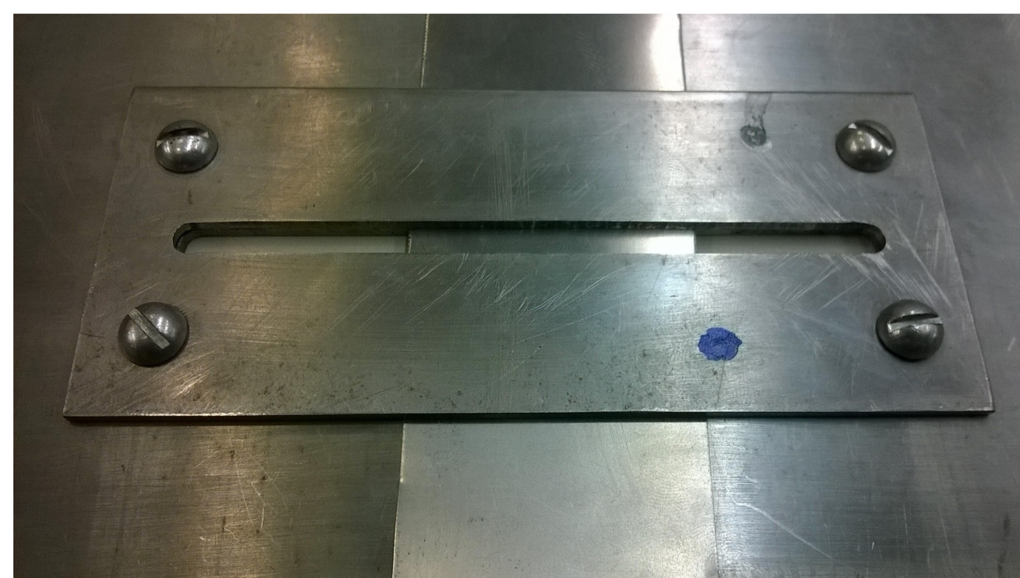
Figure 02: fixing system with the sheets positioned.
