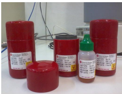
Figure 2. From left to right: ^{57}\text{Co} , ^{137}\text{Cs} and ^{133}\text{Ba} sources to the quality control tests
