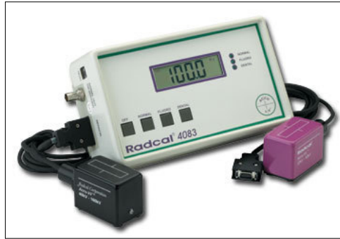
Figure 3: Accu meter Radcal KV model 4082 coupled to the sensor Radcal Accu KV 22-40 KV, Model 40x5 - Mo
