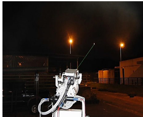
Fig. 2. Cubatão scanning lidar in operation during the sampling sequence of the flare.
