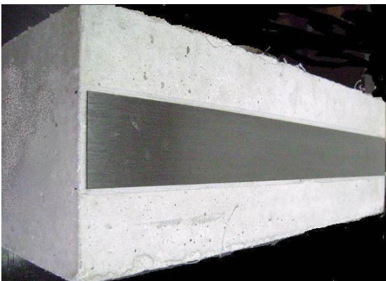
Fig. 4. Unidirectional CFRP sheet bonded to the concrete specimen.
