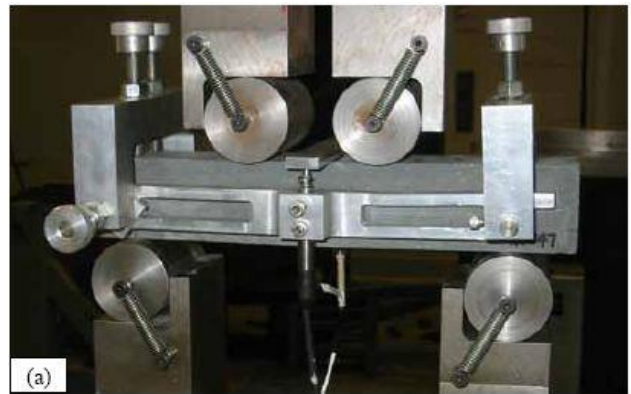
Fig. 5. Four point bending flexural test.
