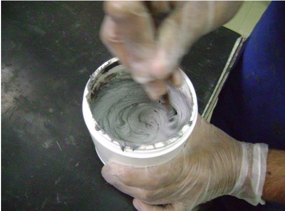
Fig. 2. Manual steering of the two-component of the adhesive.
