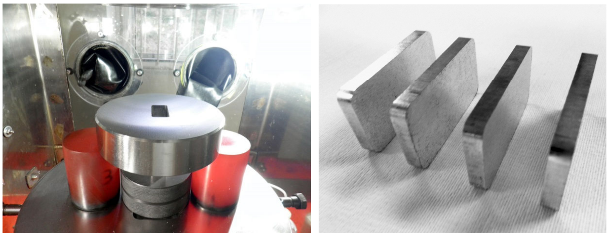
Figure 4. Photographs illustrating the pressing die (left) and the briquettes produced (right).
