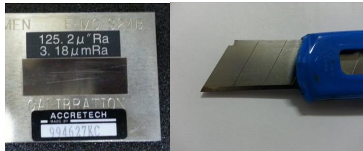
Fig. 3: Sample's photography: Roughness standard (left); Cutter knife blade (right).
