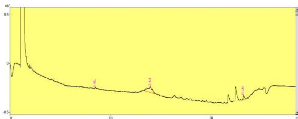
Figure 5: Chromatogram with neonicotinóides mix of 0.7 mg/L
