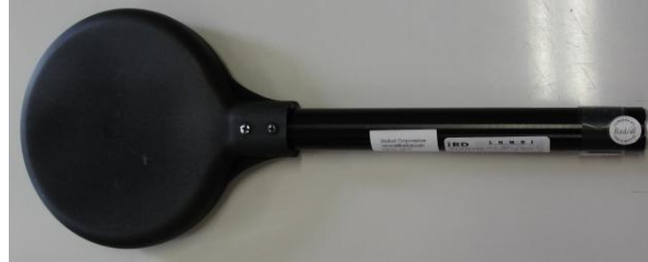
Figure 4: Radcal RC180 ionization chamber which can be used in both diagnostic radiology and radiation protection measurements.
