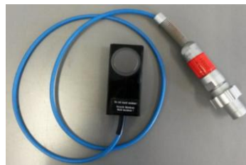
Figure 3: PTW ionization chamber, 23344 model, used in low-energy radiotherapy beams measurements.
