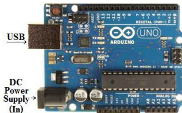
Figure 2: ARDUINO UNO board [3], employed for development of the readout module.
