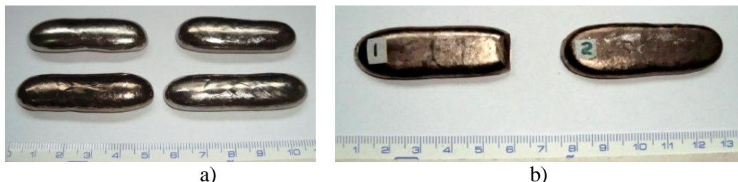
FIGURE 1. a) Ingots obtained in VAR furnace after melting Zry-4 machining chips. b) Samples 1 and 2 after hot-rolling and encapsulation removal.
