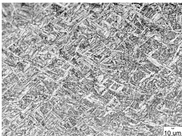
FIGURE 3. Optical micrograph sample 1 after the annealing at 850 °C and hot rolling, with characteristic morphology of Widmanstätten structure of basket weave form[11].
