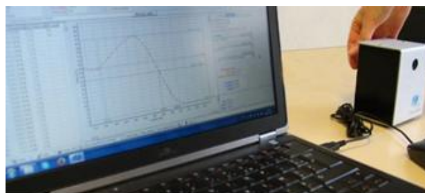
Figure 5: Dos'ASAP equipment (Aerial) measuring the strip in a continuous mode.
